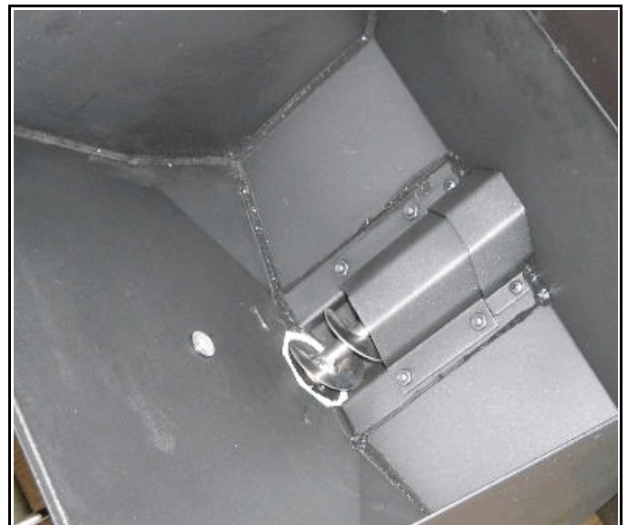
Empty hopper, auger clean out, and low fuel sensor
